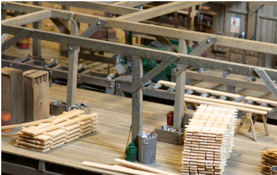
Figure 5-7 In the shipping area, lumber is piled and stickered for air drying. Coopers, cabinet makers and wainrights (carriage builders) are very particular about their lumber and normally air dry their own. Liam Hicks properly stickers lumber after milling to ensure proper air drying before the lumber is picked up by these craftsmen.
