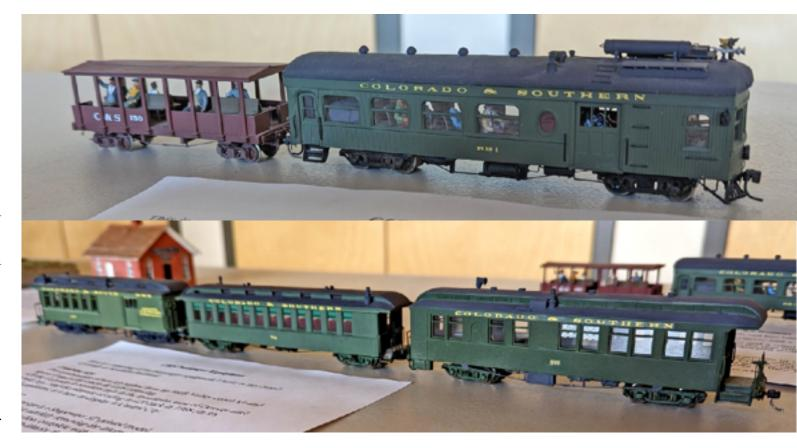
created along with inclusion of kitchen fixtures and furniture. Commercial castings were used wherever available. Things like grab irons, truss rods, steps and brake wheels were added. I chose to use Blackstone trucks and Kadee couplers. Microscope slides were used for the windows, model is covered with Floquil paints and Microscale decals.
