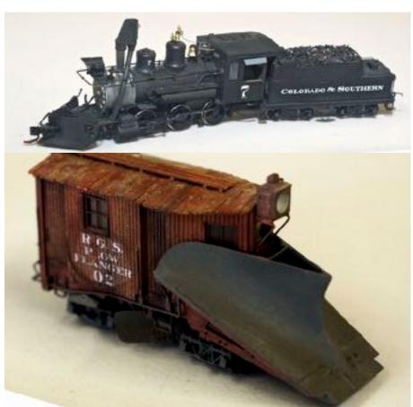
These blades were also extended higher on the outer edges resulting in an appearance that resembled the wings of a butterfly. Here Number 7 sports a Butterfly Plow and if you look closely, a Priest flanger blade mounted on the front of the pilot truck.
