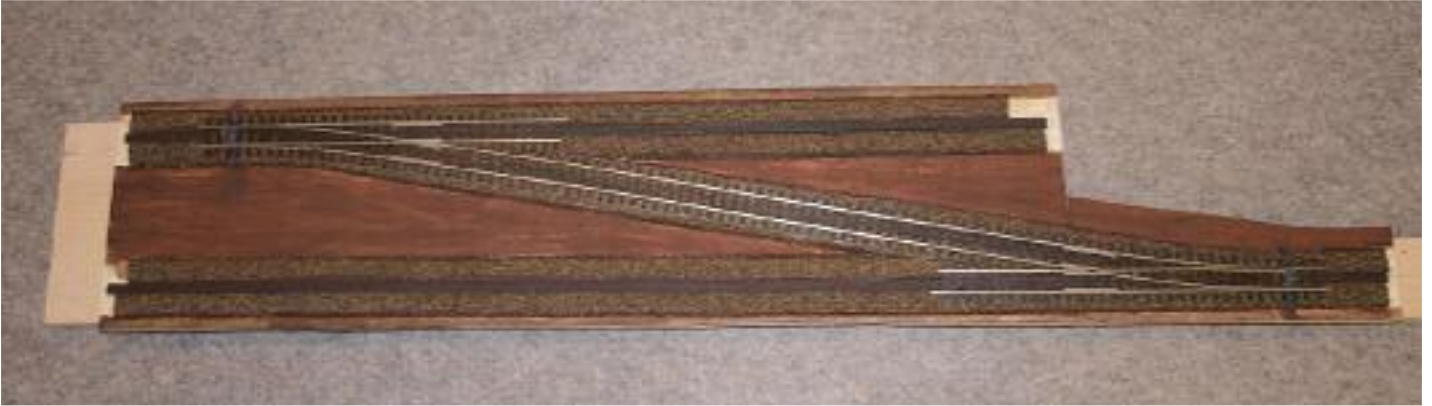
No. 6 cross over fully pre-assembled and ready to be installed on the layout. Photo: Peter Nesbitt
