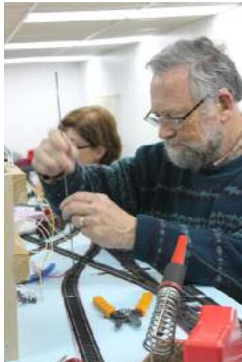
Photo 4 (Top Right): Ed, one of our new members, dove quickly into wiring the layout after receiving instructions from Peter. Track feeders were installed on each section of track to ensure future trouble free operations.
