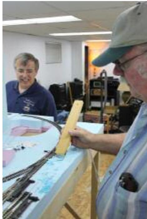
Photo 2 (Right): Paul was in charge of the Styrofoam carving (note the heavy duty home built nichrome cutter) and installing the switch stands.
