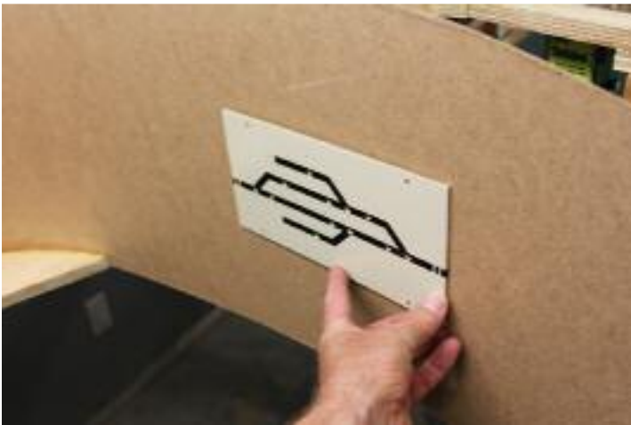
The panel outline is traced onto the fascia where it will be located.
