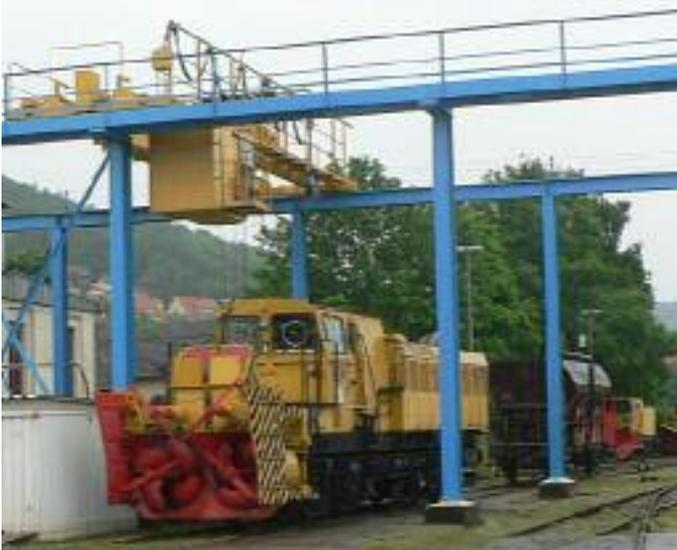
Self propelled rotary snow blower. The top portion with the rotary blower can rotate on the frame to eliminate the need for turning facilities.
