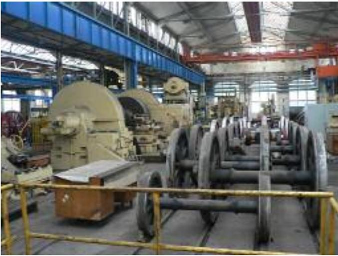
Wheel lathe and wheelsets before (front) and after (rear) rework
