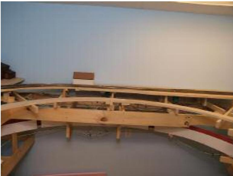
First up was the mainline west from Renfrew to Eganville, a distance of just over 63 feet at a continuous grade of 2.2 per cent. Again this was flex track on cork roadbed glued to  $\frac{3}{4}$ " plywood. There are a number of curves on this trackage as it winds around the outside of the room and over the gate at the entrance of the room.
