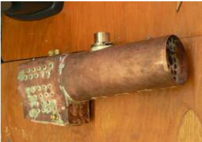
John Stewart takes the award for the heaviest model – a boiler for a 3.5 in (1:16 scale) steam locomotive. (Bottom left) John has scratch built this boiler over a number of years and is now ready for its pressure test at 200 pounds / sq in. John had hand formed the copper boiler and silver soldered the pieces together. The boiler even sports a steam super heater. Update: John has since identified that the boiler did pass the pressure test with flying colours!
