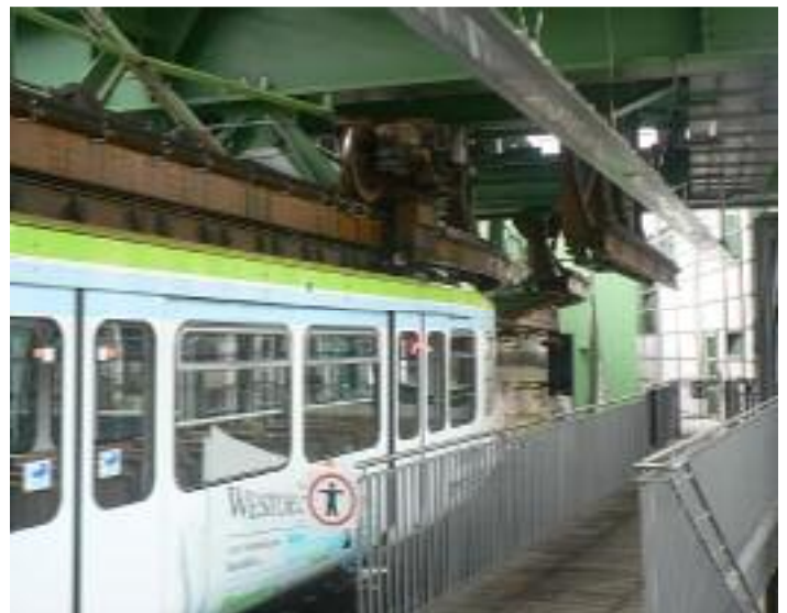
The train hangs off the top of the rail. Here the train has a choice between going straight into the car barn or to loop around and return to the other end of the line.
