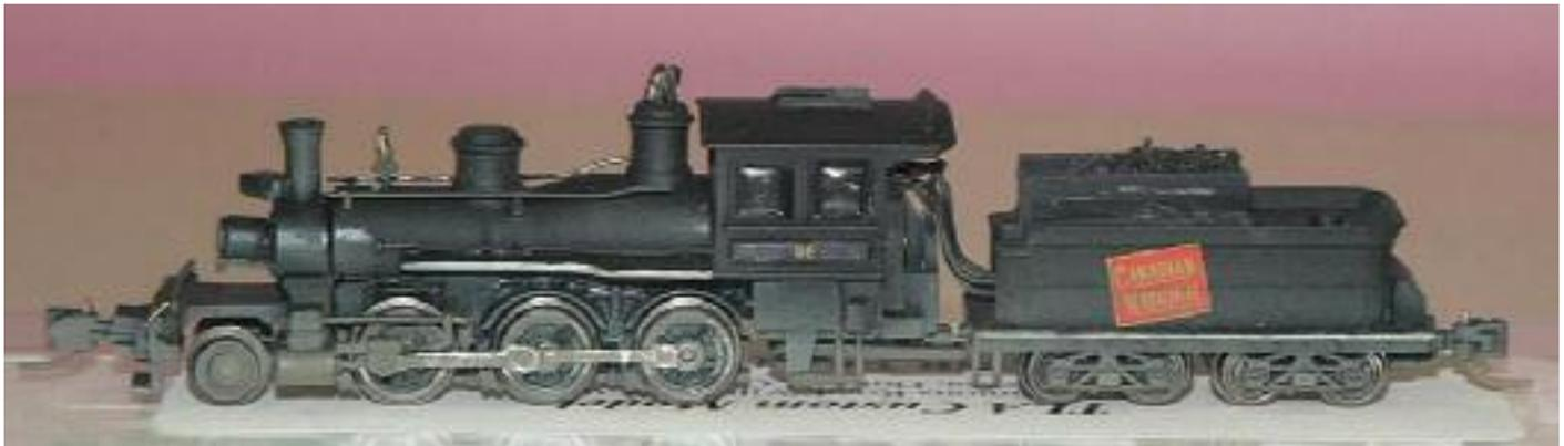
John Licharson dropped in and displayed his summer project, which he describes as “comic relief”. John modified an Atlas N-scale 2-6-0 to closely represent a CNR prototype by applying front coupler, a step pilot, new headlight, new stack, and cleaning up the lines of the tender. He also installed a Lenz decoder and other stuff that he forgot.
