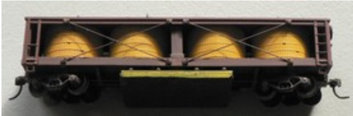
Figure 1: (Top) The magnet under this Pickle Car sweeps the tracks from metallic debris.
