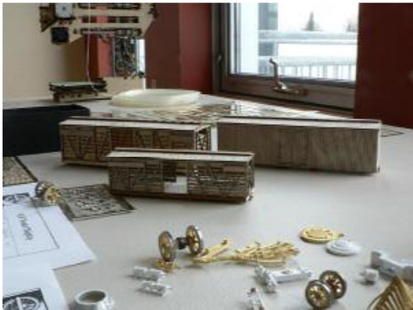
Bottom: This assortment of carbodies and detail parts are the masters for a series of S and O scale models by Bill Meredith
