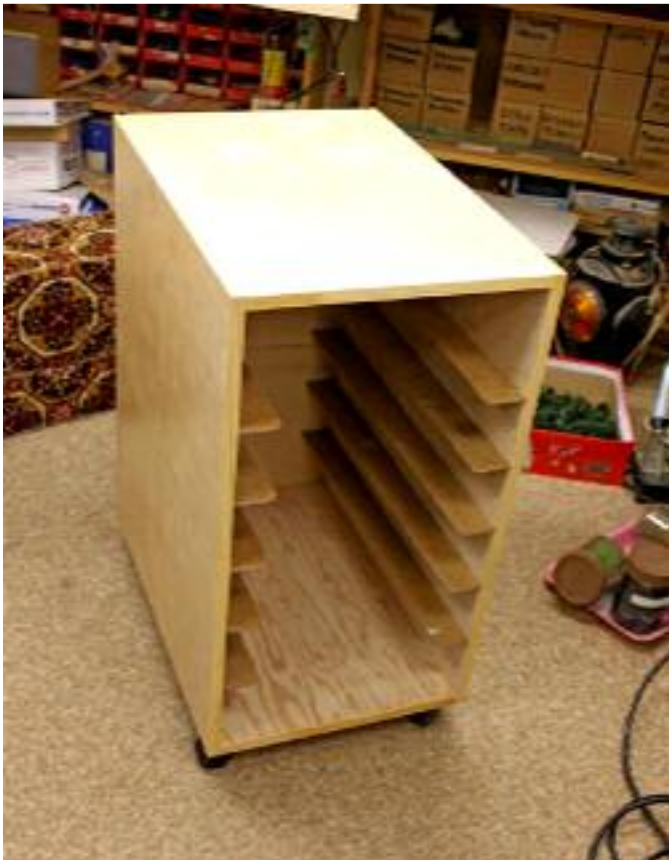
Bottom - The finished model cabinet complete with the masonite shelves and mounted on casters.
