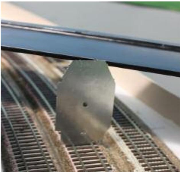
Photo 4: Track clearance is slightly less than the NMRA standard.
