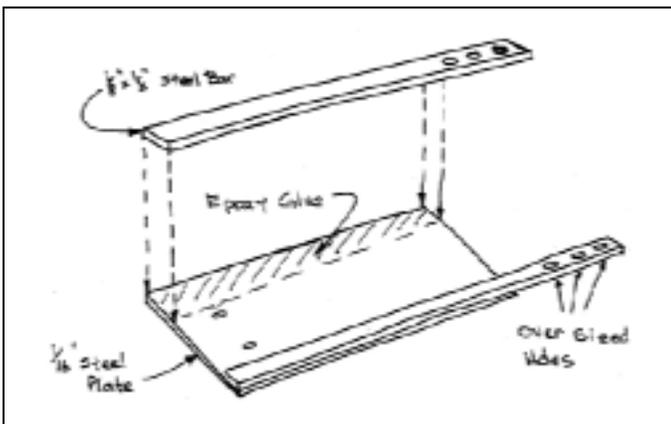
Diagram 1: The bridge is comprised of a 1/16" steel deck with two 1/8" x 1/2" steel bar stock glued on.
