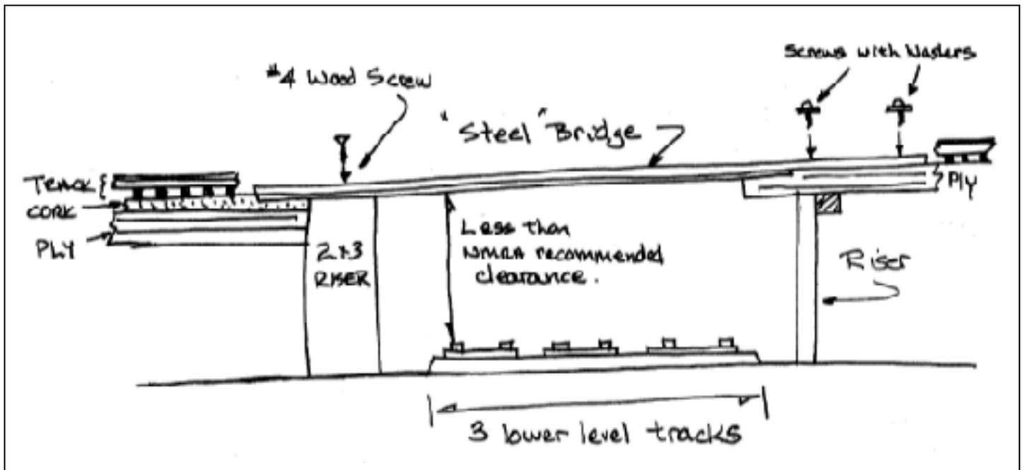
Diagram 2: Side view of the installation demonstrating the mounting arrangement.
