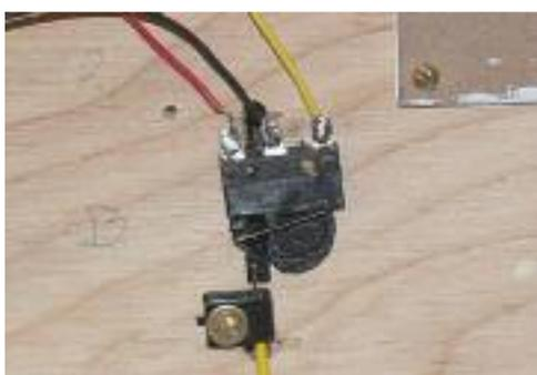
A micro switch is a much cleaner solution to provide frog power with the correct polarity.
