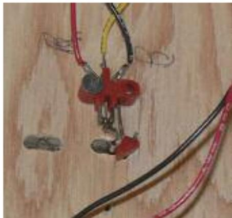
Micro-switch linked to the throw bar for changing polarity on Peco electrofrog turnouts.
