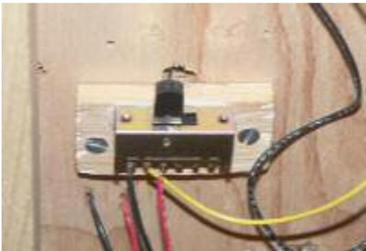
Slide Switch actuator, the coat hanger is not yet installed.
