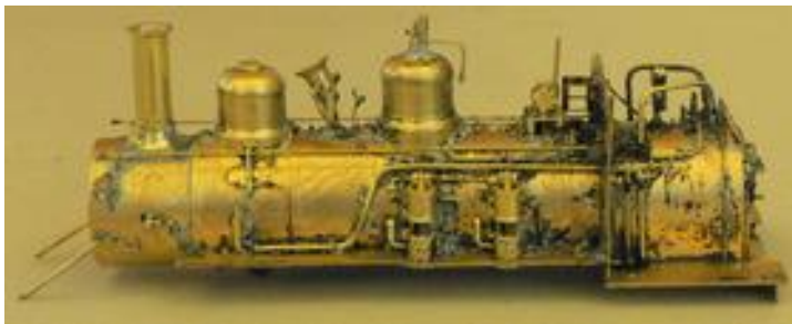
Photo 3 (Below): C&S 537 conversion from an Sn3 C21 brass locomotive.
