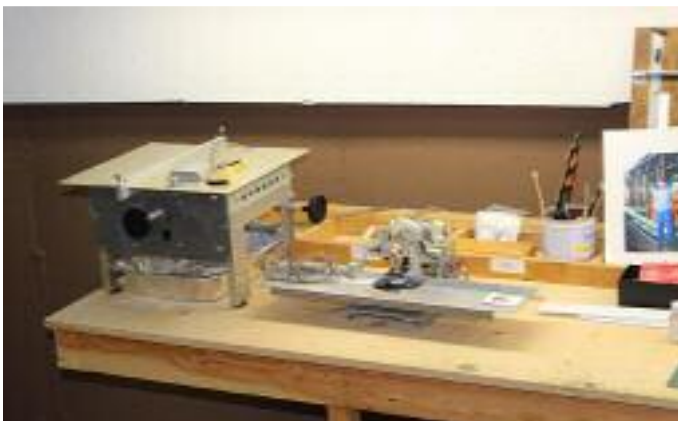
Figure 2 (Bottom): Miniature table saw and chop saw build from recycled computer components.
